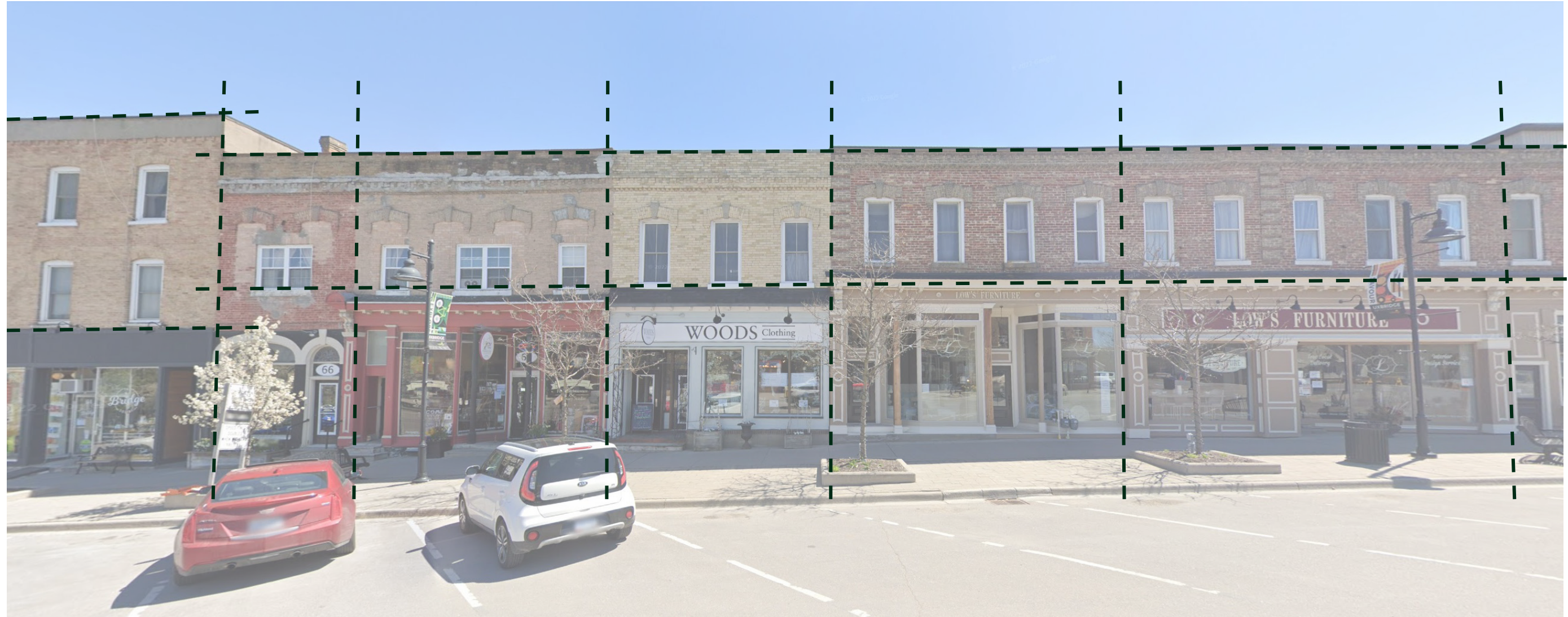
Elevation of Brock St. showing strongly articulated building bases, prevailing 2-3 story street wall expression, and rhythm of storefronts, typically comprising 2-4 window bays.
