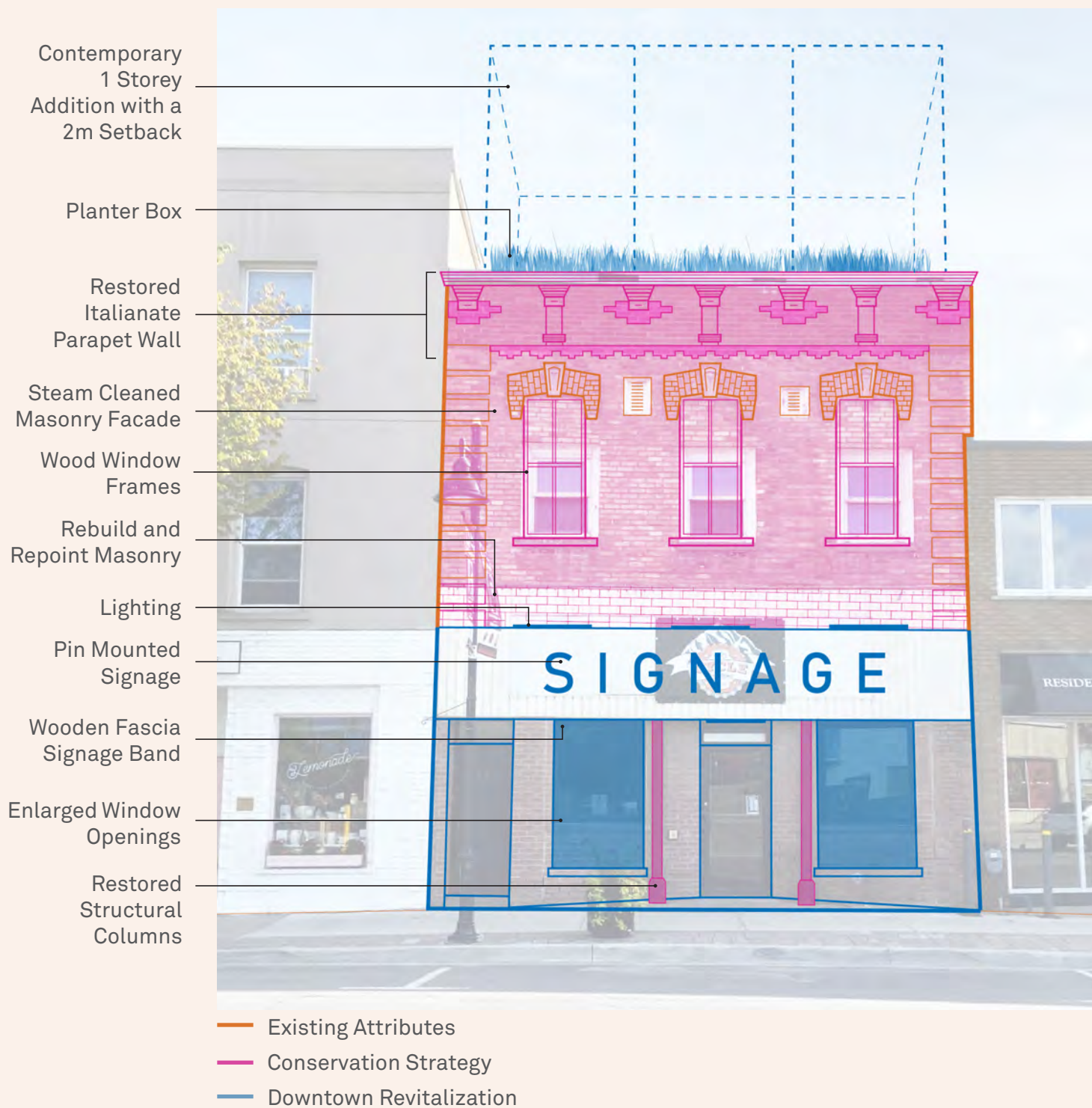
Figure 22 Diagram showing a conservation strategy for heritage building with potential addition envelope at 28 Brock Street West. Diagram created in 2025.
