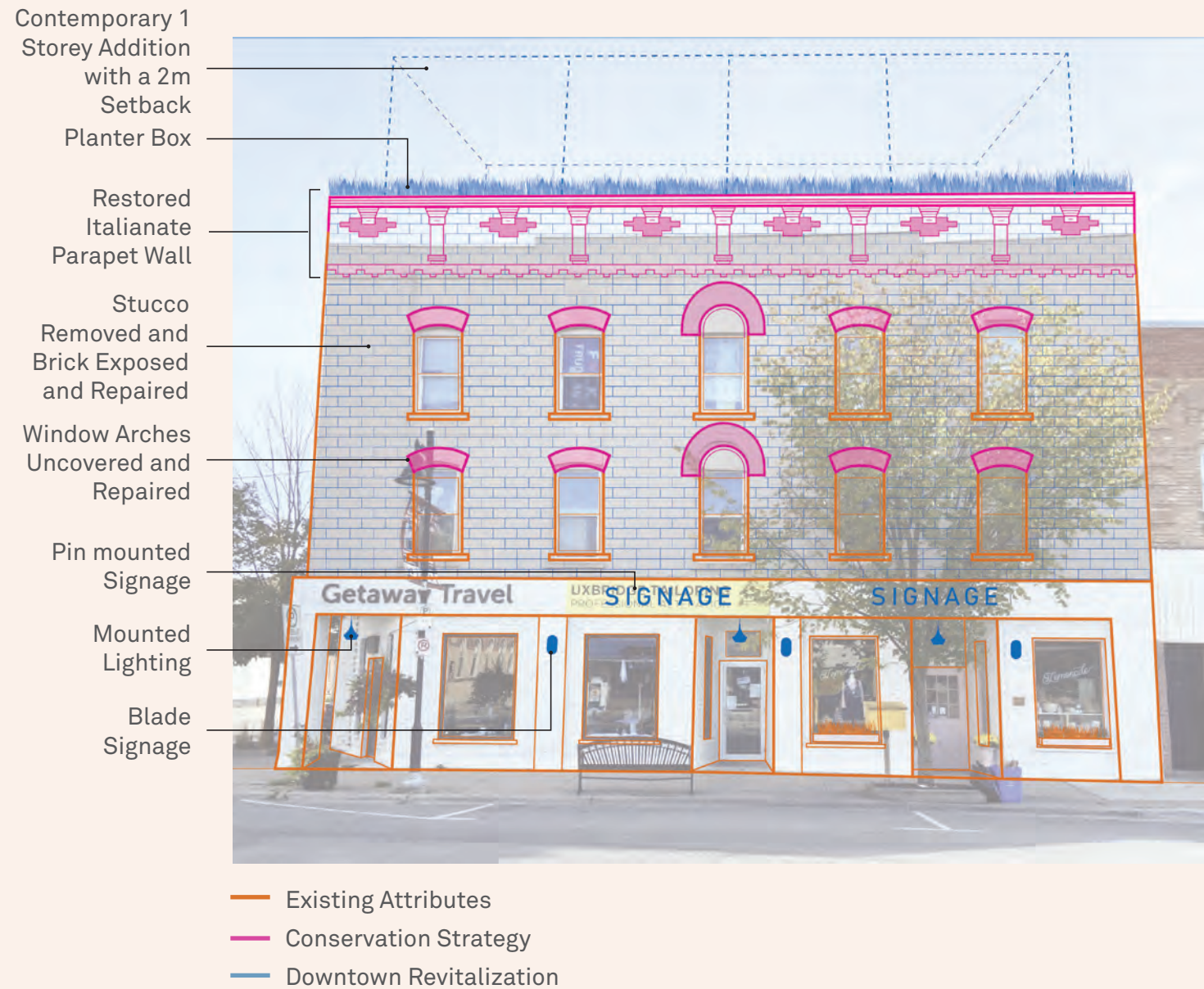
Figure 23 Diagram showing a sympathetic renovation with potential addition envelope at 22-26 Brock Street West. Diagram created in 2025.
